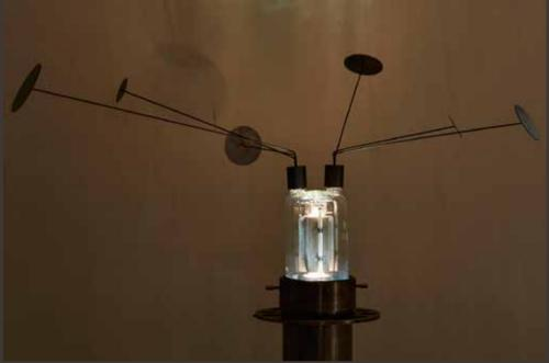
4P55: Pentode for transmitter tube, uniquely developed in Japan based on NHK's request,
