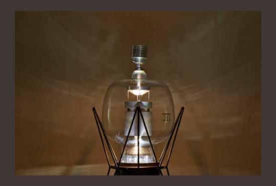
T800-1: Triode for high frequency welding machine, THOMSON, France
