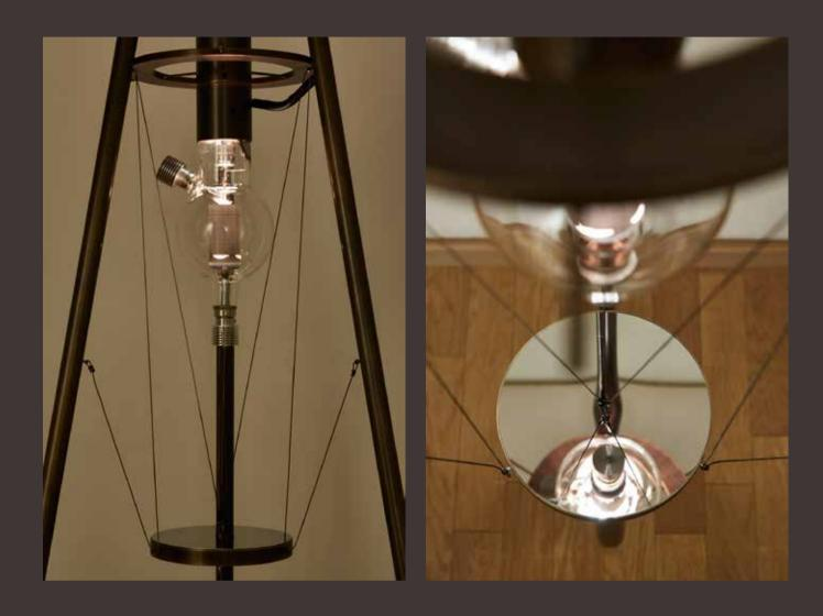
5T31: Triode for broadcasting transmitter or industrial high-frequency generator,
