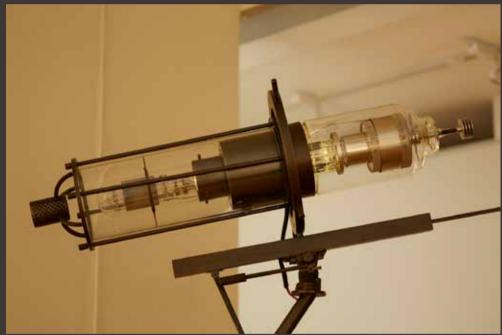
5G57P: Pulse modulation tube for large-scale radar, JRC, Japan
